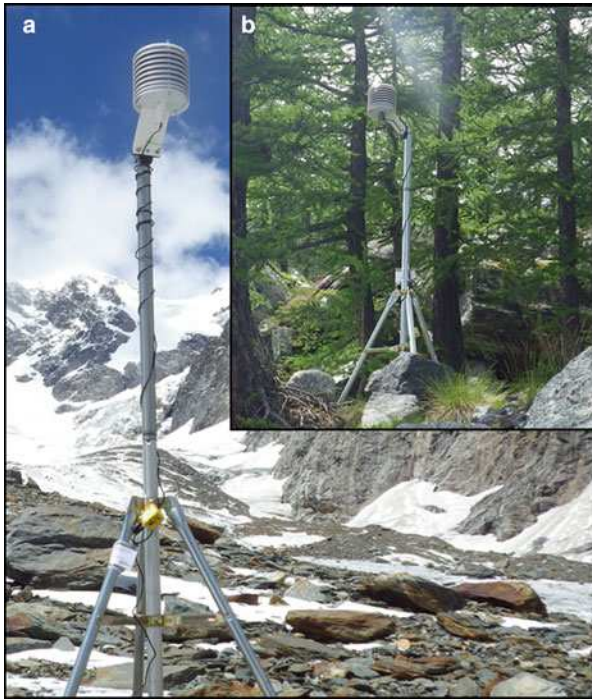
Fig. 2. (a) TT13 as an example of the temperature station in the field (image taken 14:20, 30th June, 2014) and (b) OG station and ground conditions.
