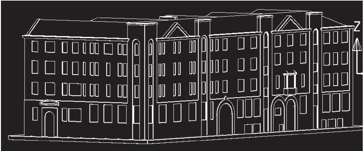
Figure 7: Using co-planar surfaces and creating sharp edges from curves in the model in Figure 6, the CAD model below is developed using Polyworks modeller and Microstation software
