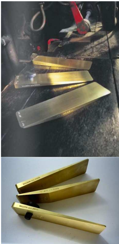
Figure group 1. Tradesman's Wedges. The wedge is one of six simple machines; a simple machine is a mechanical device that changes the direction and magnitude of a force and has been used for millennia.
