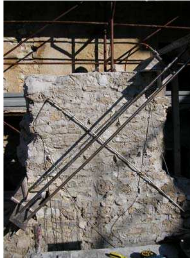
Figure 7. The diagonal compression tests
