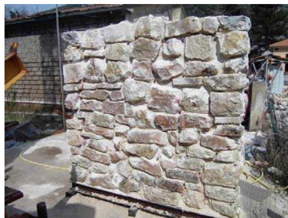
Figure 10. The second panel subjected to flexural tests
